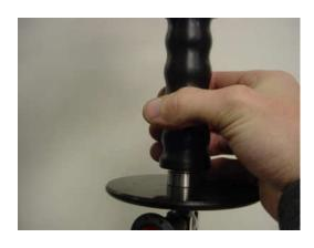
If you relieve the carpus and give small, precise movements with your fingertips the hoist will move with a low and controlled speed, this grip is good when handling fragile goods, fitting the lift object when assembly, fixtures e.t.c.
