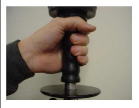
Using the whole hand gives big movements and therefore a high lifting speed of the hoist, this grip can be used when handling not fragile goods.
